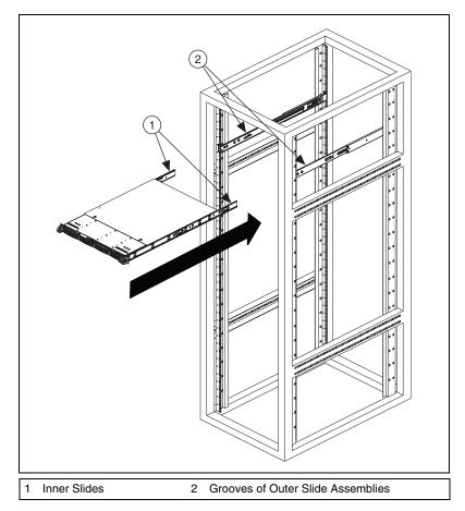
Figure 2-4. Installing Inner Slides into Outer Slides
